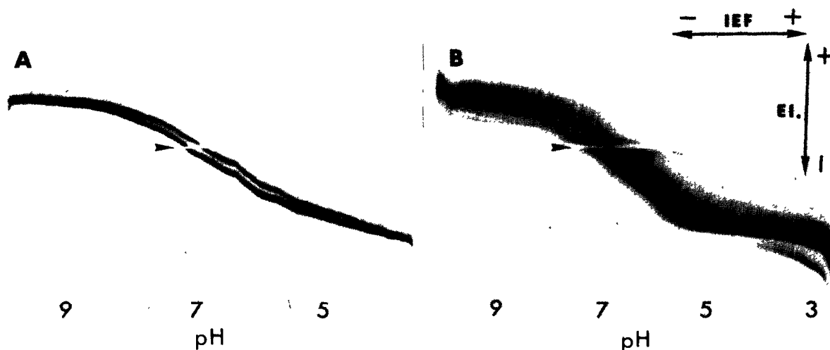
Fig.1. Titration curves of a mixture of HbA and HbA-G6P complex. Gel slab (2 mm thick): 7% acrylamide, 2% Ampholine pH 3.5-10, 5 mM Asp, 5 mM Glu and 5 mM Lys. First dimension: 90 min run in the LKB 2117 Multiphor chamber by delivering 15 W with an LKB constant wattage power supply. Coolant temperature: 2°C. Second dimension: 20 min run at 800 V, 10 mA with a sample load of ~200 \mu g protein. Staining: colloidal dispersion of 0.1% Coomassie brilliant blue G-250 in 12% trichloroacetic acid and 1 N \text{H}_2\text{SO}_4 as in [9]. (A) Red blood cell lysate incubated for 4 h with a 5-fold molar excess of G6P in the deoxyHb state; (B) same as (A) except that the sample was then treated with \text{NaBH}_4 and run for 35 min. Notice that in this case the HbA-G6P complex is now ~70% of the total. The two arrows and positive and negative symbols represent the direction and polarity of isoelectric focusing (IEF) and electrophoresis (EI.). The arrowhead indicates the application zone (i.e. the zero mobility or isoelectric plane). In both cases, the joining of the two curves around pH 4 is due to instability of unliganded HbA at this pH.
